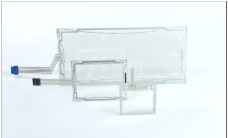
Five-wire touchscreens range from as small as 2.4" to as large as 23". (Shown are 7" off-ratio, 3.9" and 2.4" sizes)
