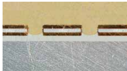
Bergquist has the ability to laminate heavy copper up to 5 oz. (175µm) on the internal layer utilizing a thicker deposit of HT dielectric.
