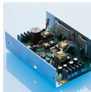
This application uses Sil-Pad to isolate the mounting brackets from the assembly frame.
