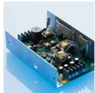
This application uses Sil-Pad to isolate the mounting brackets from the assembly frame.
