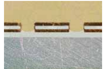
Bergquist has the ability to laminate heavy copper up to 5 oz. (175µm) finished on the internal layer utilizing a thicker deposit of HT dielectric.
